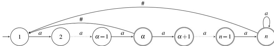
**Fig. 6.** The incomplete  $n$ -state dfa  $A$  over  $\{a, \#\}$  with  $\|P(L(A))\| = \alpha$ ;  $1 \leq \alpha \leq n-2$ .
