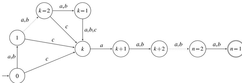
**Fig. 5.** The minimal incomplete dfa over  $\{a, b, c\}$  accepting a finite language meeting the upper bound on the projection onto  $\{a, b\}$ ;  $k = \lceil n/2 \rceil - 1$ .
