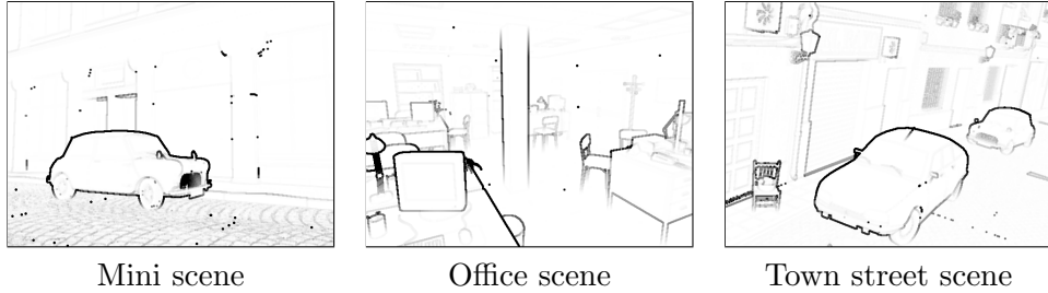
Figure 4.3: Second gradients of \frac{1}{z} = f(u, v) represent the strength of discontinuities. Each in the 3rd image of the sequence, the magnitude of f is represented by grey-values, normalised to the images average, scaled by i = 5 and dilated for visualisation purposes. White represents f = 0 , black f \geq \frac{1}{5} .
